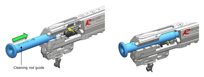
To use a brush, you will have to remove the cleaning rod guide socket. Insert the cleaning rod (without brush) in the socket and then screw the brush onto the cleaning rod.
