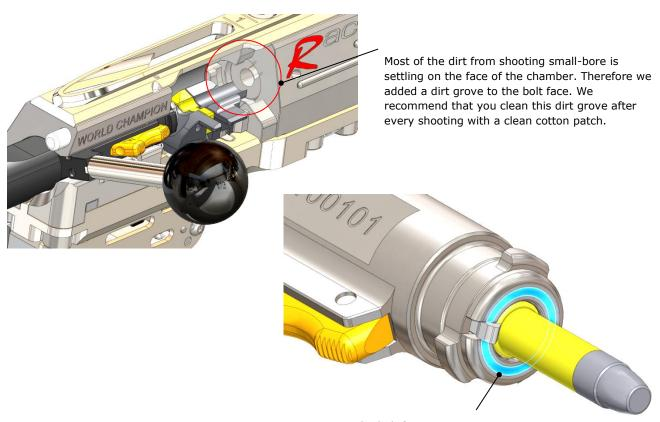
Dirt groove on the bolt face.
