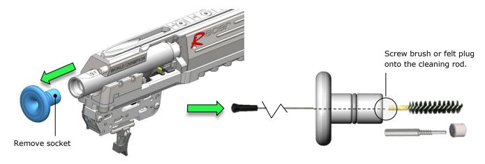
Push the socket with the brush attached, into the cleaning rod guide.
