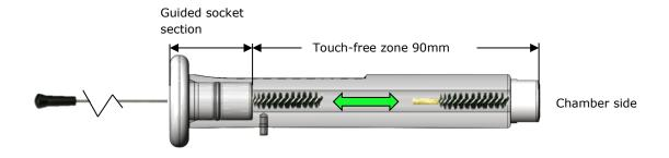
The cleaning rod guide is equipped with an O-ring. The O-Ring seals the space between the clearing rod guide and the chamber face during cleaning. The O-ring is important to prevent dirt from entering the action.
